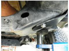
Now you can place the rock sliders on jack stands and align them with the holes from the L-Bracket Frame mount. There are CNC cut holes to make space for existing bolts and plugs on the frame from the factory.
