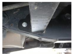
Next, drill a 3/8" hole in the rear and insert a hex head bolt with flat washers and locknut. You will need to use a 9/16" wrench/socket to tighten all the 3/8" hex head bolts to 44 ft/lbs (pictured left).
