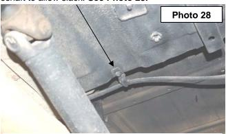
Bend bracket down to allow for slack
