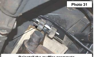
Reinstall the muffler grommets
