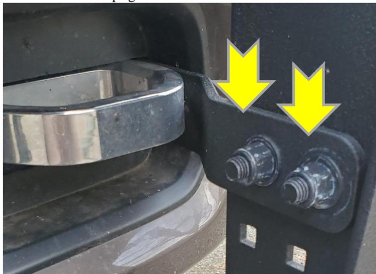
7. Slide lower mounts into place through the cuts in the spoiler. Using (4) 3/8 bolts, (8) washers, and (4) nylock nuts from hardware kit #215, bolt lower mounts to the truck. Use (4) carriage head bolts, washers, and nylock nuts from hardware kit #208 to fasten lower mounts to the grille guard. The mounts should sit to the inside of the grille guard.
