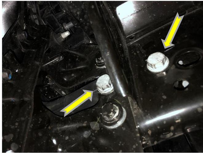
7. Remove the tow hooks through the front of the bumper and set them aside along with the hardware.
