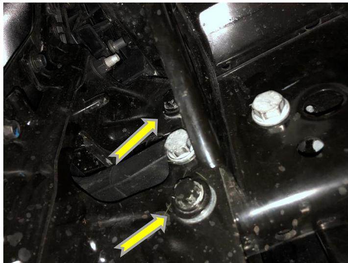
9. Locate the push clip on the bumper spoiler directly under the bumper mount. Make a mark on either side of the clip approximately ½". Measure Trim along this mark with your cutting tool of choice 4" to allow the lower mounts to pass through.
