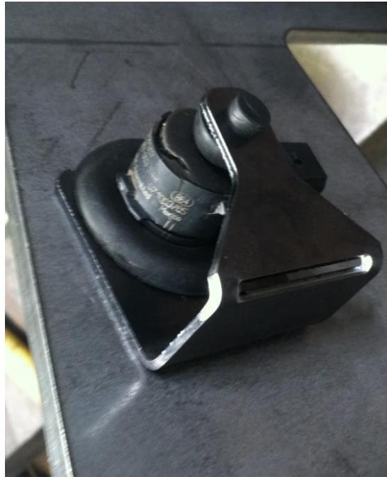
3. Slide the bumper forward enough to slide the lower mounts into place. The notch on the mounts goes towards the bottom.
