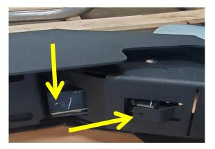
4. Install Hammerhead BSM plastic covers. They bolt in to the step using a carriage head bolt and nylock nut.
