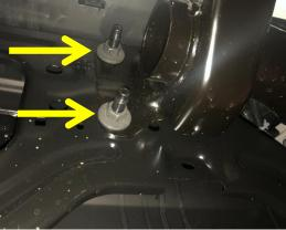
5. Using trim tool, remove one plastic retainer attaching wire loom to bumper. (arrow) Leave module plugged in. Unclip module out of bumper and allow it to hang down.
