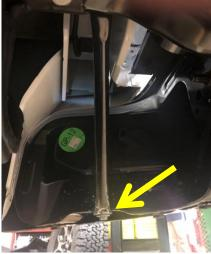
4. Using 18mm socket or wrench, remove two nuts attaching OE bumper to receiver hitch. (both sides)
