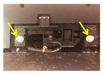
7. Using 21mm socket, remove nut attaching side brace to frame. Remove brace and replace nut.
