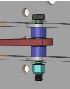
5. Using a 9/16: socket, install the 3<sup>rd</sup> brake light bracket and the Spare Tire Adapter onto the Spare Tire Carrier as shown. Use the 4 carriage head bolts, washers, and nylock nuts from hardware kit #152. The brake light bracket and spare tire adapter are adjustable vertically for different size tires. (35" in the lowest position, 40" in the highest position.) IT IS VERY IMPORTANT TO TIGHTEN THESE BOLTS TO SPEC OR RISK HAVING YOUR SPARE TIRE FALL OFF THE VEHICLE
