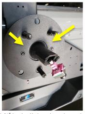
8. Route the Camera and 3<sup>rd</sup> brake light wires through the hole shown below.
