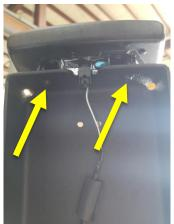
10. Using a 9/16" socket, install the cups on the Spare tire Carrier using two carriage head bolts, washers, and nylock nuts as shown below. Do NOT tighten bolts yet.
