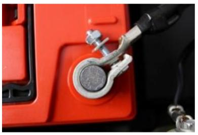
17. Remove the factory post clamp bolt, and insert the provided longer post clamp bolt, the factory square washer, and one provided nut. Tighten the post clamp.
