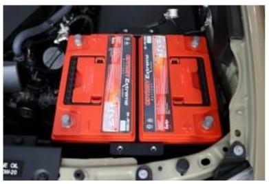
7. Install the aux battery first. Shift the tray as needed to get the battery to slide all the way towards the fender, clearing the headlight assembly at the front corner. Install the cranking battery next, with the posts towards the engine. Adjust the position of the tray so the battery does not interfere with the oil fill cap.
