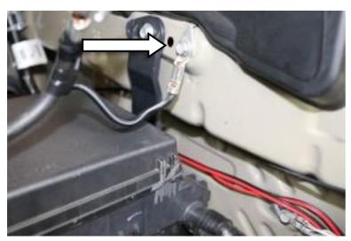
3. Use a 10mm socket to loosen the bolt for the ground wire on the inner fender. Rotate the wire 90 degrees for better clearance for the new batteries, and tighten the bolt.
