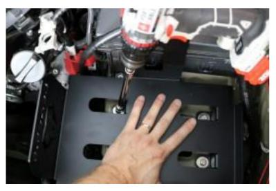
13. Drop in the provided stainless bolts with washers into the well nuts.
