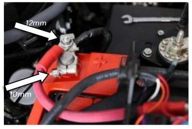
19. Tighten the factory positive post clamp with a 10mm socket. Install the red wire under the factory 12mm nut as shown.
