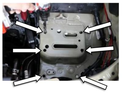
10. Drill the holes using a 25/64" drill bit. Note: It is critical to use the correct size bit so the nutserts will clamp properly.
