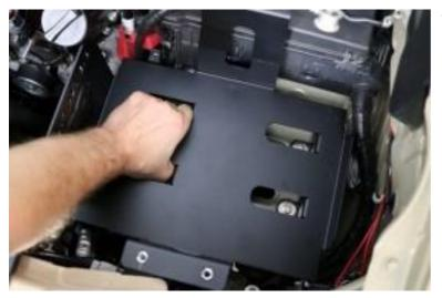
14. Double check your alignment marks. Adjust the position as necessary, then tighten all 6 bolts. The base of the tray should be very sturdy and not move at all.
