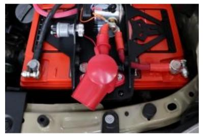
20. Tighten the other 2 post clamps with a ½" socket or wrench. Be careful not to bump the factory sheet metal when tightening the positive post clamp.
