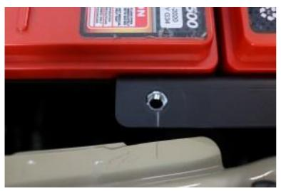
8. After verifying clearance by the oil fill cap, the fuse box wires, the headlight assembly, and the stamped raised areas by the lower legs, make an alignment mark with a pencil on the tray and the factory sheetmetal. Carefully remove the batteries so that we can center punch and drill holes to secure the tray. Use the alignment mark to ensure the tray does not move.
