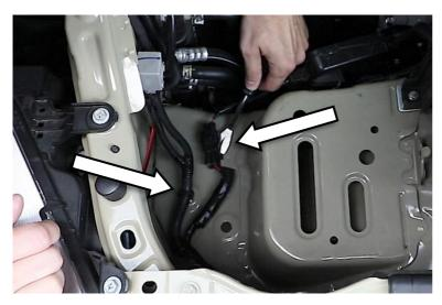
5. Use a pry tool to move these 2 factory wires to make room for the new tray legs. Disconnect the plug now for easy access for your center punch later.
