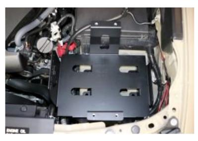
6. Drop the new tray in place. Note it will be a very tight fit in all directions. To the rear it will touch the fuse box support leg. It should clear the oil fill tube by a few millimeters. Make sure all 6 legs sit flat on the factory sheet metal. Avoid the raised stamped areas by the lower 2 legs. Ensure the tray does not touch the radiator hoses at the front corner. If necessary, gently push the hoses out of the way.
