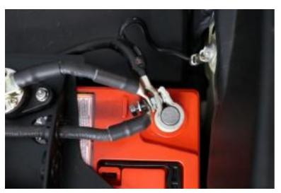
18. Place the lid on top of the batteries. Put the short ground wire onto the post clamp first, then the longer ground wire, the round washer, and nut. Tighten the nut to secure the ground wires.
