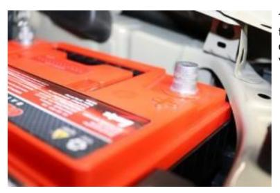
15. Reinstall your batteries. Ensure they both sit flat and level with each other. The front corner will be very tight to the radiator support.
