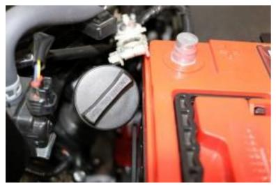
16. You should be able to remove the oil fill cap with no interference. If necessary, reposition the tray for clearance.
