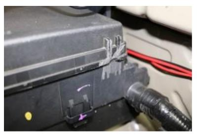
4. Use a cutoff wheel, air saw, or similar to trim off the latching tab on the front of the fuse box and lid. This will allow extra room for installing the batteries. The lid will still stay attached securely.
