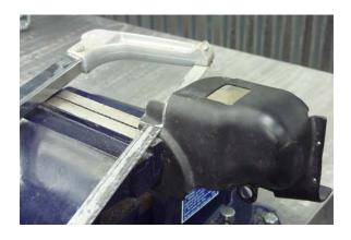
Step 5 Secure the cover in a vice and along the marks using a hacksaw (or cut off wheel).
