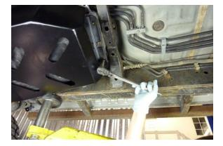
Using a 12 mm socket, tighten all four bolts.
