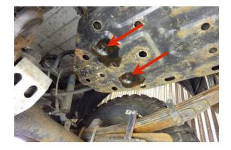
Step 3 Spray the (2) rear bolts with penetrating oil.
