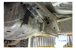
Remove the driver side front bolt using a 12 mm socket.
