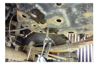
Step 6 Remove the driver side rear bolt using a 12 mm socket.
