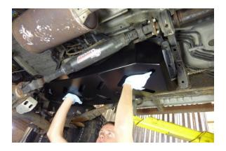
Step 11 Position the Low Range Off-Road Gas Tank Skid Plate and align the bolt holes.
