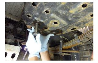
While supporting the fuel tank protector with one hand, remove the driver side rear bolt.
