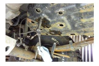
Step 7 LOOSEN, but do not remove, the driver side rear bolt using a 12 mm socket.
