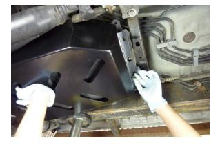
Have an assistant support the gas tank skid plate while you start the driver side front bolt. Just 3 or 4 turns.
