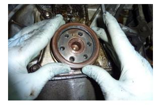
Orient the seal such that the girdle spring is facing toward the engine and position it over the crankshaft.
