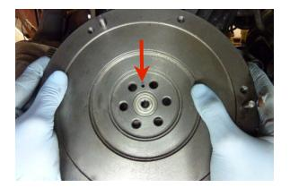
Step 20 Orient the locating hole of the flywheel so it aligns with the locating pin in the crankshaft.
