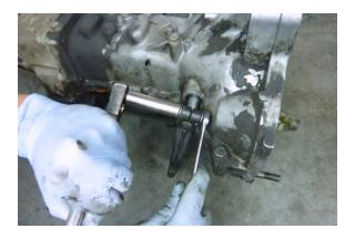
Step 39 Tighten the pinch bolt and nut to 7.5 to 11.5 ft. lbs.
