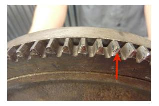
Inspect for tooth wear on the starter ring. If wear is excessive it is best to replace the flywheel.
