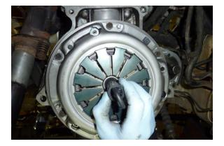
Continue pushing the alignment tool inward until it has engaged the clutch disc as well as the pilot bearing.
