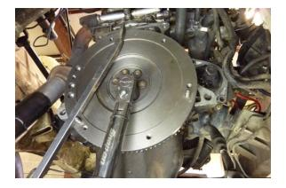
Step 22 Lock the flywheel using a pry bar and torque the bolts 41.5 - 47 ft. lbs.
