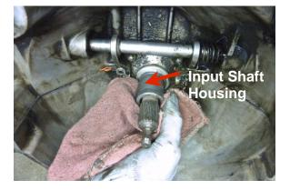
Clean the input shaft housing and inspect for wear. The housing should be replaced if it has grooves, cracks or any uneven surfaces.
