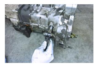
Step 33 Remove the clutch release lever.
