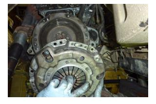
Step 3 Set the clutch cover and clutch disc aside.
