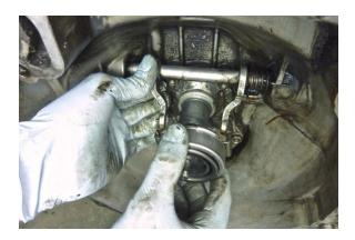
Step 34 Rotate the release shaft toward you and remove the clutch release bearing.
