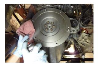
Step 23 Clean the machined surface with brake cleaner and a cloth.
