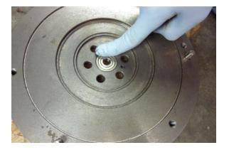
The bearing should be flush with the flywheel.
