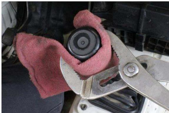
*Picture showing hard-to-remove shift knob removal.*
