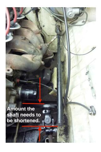
With the rag joint eliminator installed, the steering shaft will be too long. It will need to be shortened or collapsed. Estimate the amount that the steering shaft needs to be collapsed by temporarily installing the steering shaft in the universal joint up at the firewall and measuring at the rag joint end.
