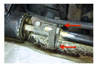
Disconnect the rag joint from the rag joint flange by removing the (2) rag joint bolts using (2) 12 mm combination wrenches.
