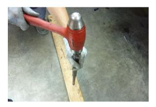
Collapse the steering shaft by placing the spline end on a piece of wood (to protect the splines) and striking the rag joint end with a hammer as shown.
