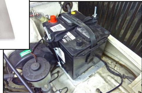
Our Dual Battery Bracket will also accommodate a larger battery. The dimensions of the battery shown here is Height = 7-3/4", Length = 8-1/2" and Width = 6-3/4". We do not supply the battery hold down kit for this battery, but it is readily available through most auto part supply stores.
