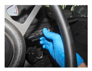
Turn the ignition key to ON and the wiper switch to LOW. Make sure the wipers sweep correctly and stop in the correct PARK position when turned off.
