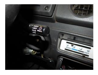
Turn the ignition key to the ON position and turn the wipers to LOW. several wiper sweeps, turn the wipers OFF. The wipers should now be in the PARK position.
