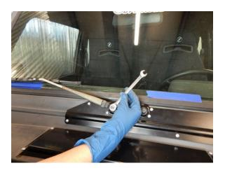
Step 20 Once the wiper arm is positioned correctly, tighten the nut.
