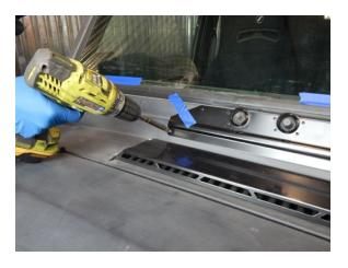
Install the second self drilling screw on the passenger side of the brace and remove the masking tape.
