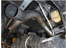
4. Place a Clamp onto the Y- Pipe inlet and install the Y-Pipe onto the Over-Axle Pipe.
