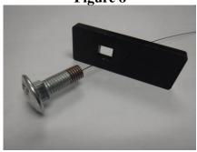
6. Thread the Bolt Leader onto the M10 Carriage Bolt, and through the Bolt Spacer.Refer to Figure 9.
