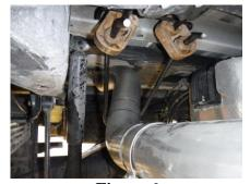
**3.** Replace the factory rubber isolators onto the truck in the original position. Using a **Clamp** install the **Over-Axle Pipe** onto the **Extension Pipe** and into the rubber isolators.
