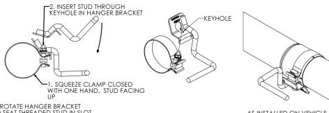
3. ROTATE HANGER BRACKET TO SEAT THREADED STUD IN SLOT. BE SURE THE NUT IS ABOVE THE BRACKET
