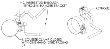
3. ROTATE HANGER BRACKET TO SEAT THREADED STUD IN SLOT. BE SURE THE NUT IS ABOVE THE BRACKET
