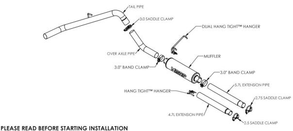
MBRP Ltd. has made every effort to ensure that all components of this system are of superior quality and properly packaged. It is the installer's responsibility to ensure that all components are present and fit together as shown. Please also ensure that all components are undamaged before removal of the factory exhaust. Finally, check that this system properly matches the make and model of the vehicle and will not interfere with previous or planned modifications.
