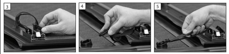
3, 4 & 5. Release the strap from the stowed position by squeezing the tabs. Attach the buckle at the bulkhead, pull the strap to take up the slack and secure the cover. Repeat this for the opposite side.
