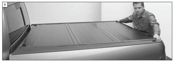
9. Test the rear latching assembly for smooth operation as this is the best indicator of the cover being positioned correctly. Be sure the latches on both sides are engaging with the cover mounting rail. *Note: If your truck is equipped with a tailgate protector, you may need to slightly raise the rear of the side mounting rails for the latches to engage properly.*
