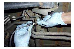
Connect the supplied flexible brake hose to the upper brake line as shown.
