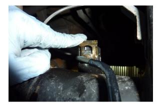
Position the bottom brake line fitting in the bracket and install the bracket lock as shown. **Caution:** Because the hydraulic brake lines were disconnected and brake fluid escaped and air entered. The brake system will not function properly until a procedure called "Brake System Bleeding" is performed. This procedure will be explained at the end of these instructions.
