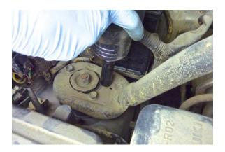
Step 30 Disconnect the passenger side cross brace using a 14 mm socket.
