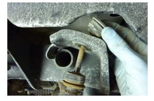
Disconnect the upper shock absorber by clamping the upper end of the shock stud with vice grip pliers and turning the nut with a 14 mm box end wrench.
