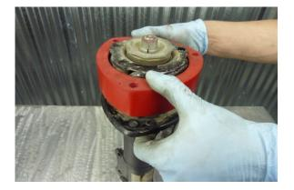
Step 40 Install the strut spacer on the top of the strut and align the holes.
