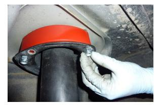
Step 44 Install the nuts from the bottom.
