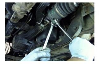
Disconnect the inner end of the drive axle by removing (3) bolts and nuts using two 14 mm box end wrenches.
