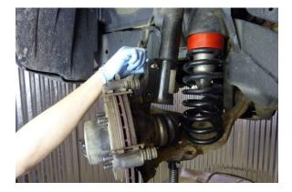
Align the upper hole in the steering knuckle with the hole in the strut and install the strut-to-knuckle bolt.
