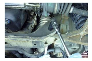
Loosen but do not remove the rear inner control arm bushing bolt by holding the bolt with a 19 mm box end wrench and tuning the nut with a 19 mm socket. (See Figure A for parts identification)
