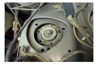
Step 33 Remove the strut by guiding it down and out of the vehicle.
