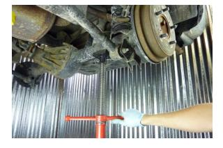
Reposition the under hoist jack stand (or floor jack) under the axle housing as shown and raise the differential back up.
