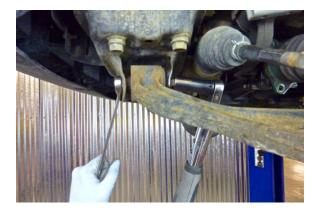
Step 65 Torque the front inner control arm bolt to 50-75 ft. lbs.
