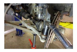
Step 68 Install the nut and torque to 22 to 40 ft. Ibs.
