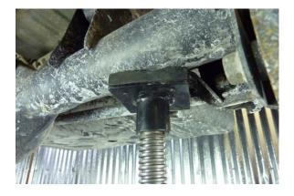
Support the rear axle assembly using an under hoist jack stand or a floor jack as shown.
