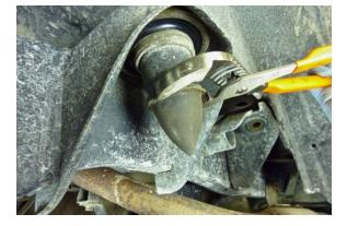
Step 110 Reinstall the bump stop and tighten.
