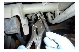
Loosen (but do not remove) the upper end of the flexible brake hose by holding the hose with vice grip pliers and loosening the flare-nut fitting using a 10 mm tubing wrench.
