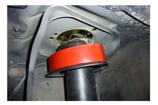
Step 41 Reinstall the strut in the vehicle as shown.
