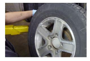
Reinstall the rear wheels and torque the lug nut to 55 ft. lbs. Don't forget the plastic lug nut caps if so equipped.
