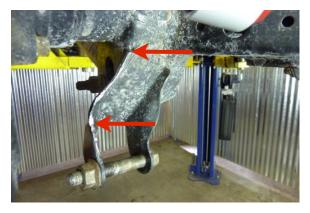
Clearancing the shock mount is done by removing the shock absorber from the vehicle. Then reinstall the lower shock mount bolt and snug the nut into place as shown. This will reduce shock mount distortion during the clearancing procedure. Using a large ball peen hammer, strike the bracket sharply in the two locations indicated by the arrows. Reinstall the shock and check for fit. Continue this procedure until the shock can be mounted without the bracket interference.
