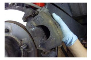
Reposition the brake caliper back in its original position over the brake pads.
