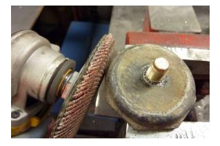
Clamp the bump stop in a vice and grind the points off as shown. This is to allow the new lift spacer to slide over the bump stop.
