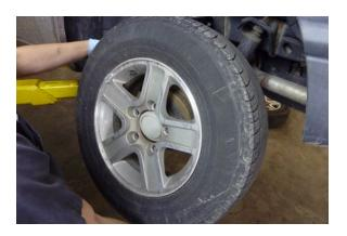
Step 89 Remove the wheel assembly.
