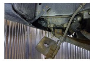
Step 19 Suspend the caliper from the body or frame using a wire.
