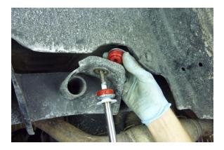
Position the upper shock stud through the upper support as shown here and install the top bushing and washer.
