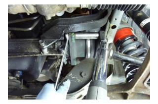
Step 70 Torque the nuts to 29 to 43 ft. lbs.
