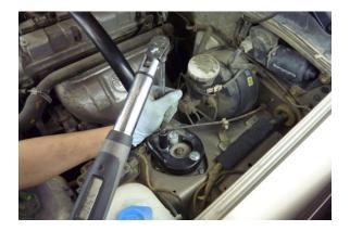
Torque all (6) cross brace bolts (passenger and driver side) to 16 to 25 ft. lbs.
