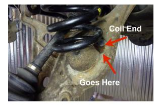
Reposition the bottom of the spring on the lower control arm. Twist the spring so the bottom coil end matches the shape of the lower control arm.
