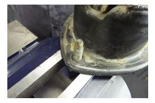
Step 34 Place the strut in a vice with the jaws open about 1/2 in.
