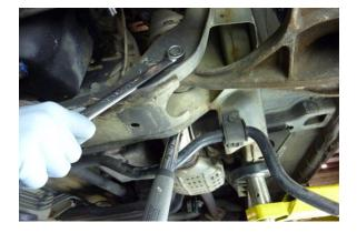
Step 66 Torque the rear inner control arm bolt to 65-100 ft. lbs.
