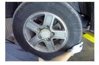
Step 6 Remove the wheel assembly.
