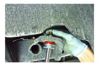
Install the lock nut with the flat side down and tighten with it a 14 mm box end wrench.
