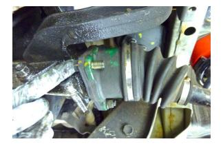
Position the drive axle and install the (3) bolts and nuts as shown.
