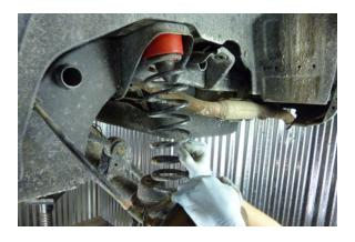
Step 112 Pull down on the differential and reinstall the coil spring. Install the top first and then the bottom.
