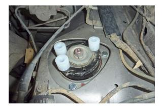
Step 80 Place (3) of the supplied spacers on top of the driver side strut as shown.
