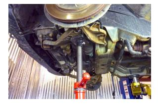
Place an under hoist jack stand (or floor jack) under the control arm and lift up until the vehicle nearly lifts off the lift (or jack stand)
