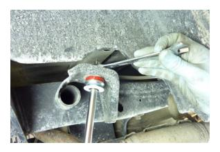
Step 119 Tighten the nut using a 14 mm box end wrench until the bushings bulge.
