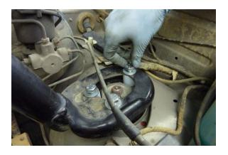
Position the cross brace and start the (3) supplied bolts on the driver side. But do not tighten them yet.
