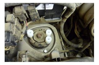
Step 81 Place (3) of the supplied spacers on top of the passenger side strut as shown.
