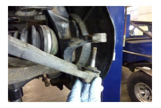
Step 67 Insert the tie rod end into the steering arm.
