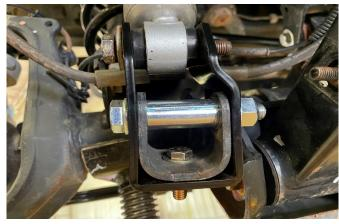
O Sleeve 93 will be used in the OE shock mounting position.
