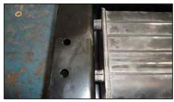
Use a 5/16" Washer and nut to attach the EVAP Canister to the new JKS EVAP Canister Skid Plate.
