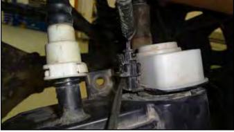
Remove the soft line either from the detector or at the connection near the frame rail going up to the fuel filler neck.
