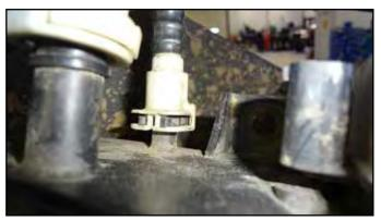
Disconnect the wire harness from the EVAP Canister on the detector (white body on the back of the EVAP Canister).
