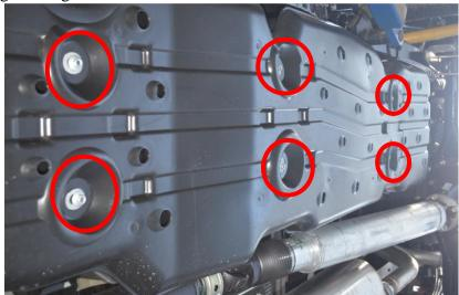
7.) Once the gas tank skid is removed, there will be enough room to get the nut plates up to the rectangular holes in the frame that align with the holes in the slider mounting plate. For the front most hole in the slider mounting plate, the same method of reaching into the frame used for the bottom front most nut plate will be used again. There is a black plastic cover on the inside of the frame in this area which can be removed in order to help align the nut plate better.
