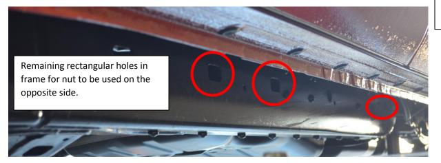
8.) Starting from front to rear, position nut plates and loosely tighten bolts, using a flat washer between the bolt head and the slider plate. Leave bolts loose until all are started. It is then okay to fully tighten bolts down once satisfied with the way the slider sits on the truck.
