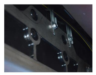
10.) After the 4 bolts in the sides of the slider mounting plate are tightened and slider is aligned properly, drill out the remaining four holes in the bottom of frame, using the slider mounting plate as a template with the 3/8" drill bit.
