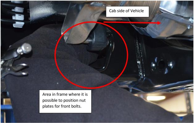
5.) Align front hole in the bottom of the rock slider mounting plate with this newly positioned nut plate. When the hole is aligned with the nut plate, finger tighten a 3/8" countersunk bolt into this nut plate through the counter sunk hole in the slider mounting plate. Leave the bolt loose for now to allow room for adjustment.
