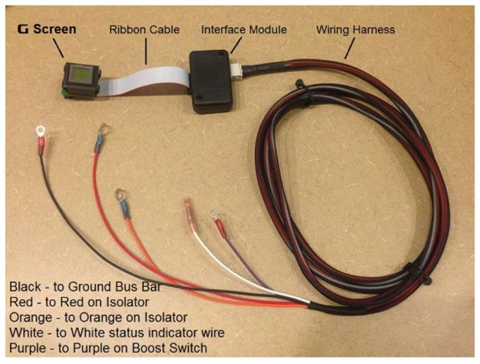
The wire harness leads are sized to perfectly line up with the components for a clean installation.
