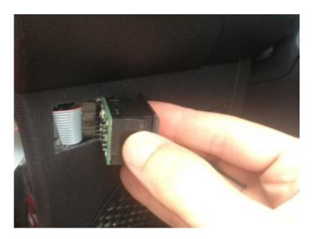
Route the ribbon cable through the hole first. Leave the ribbon cable connected to the screen during installation as it may be difficult to connect it once the screen is in place.
