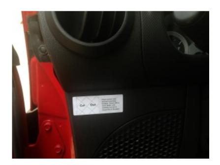
Place the template sticker where you want to mount the **G** Screen. Use an X-Acto knife or razor blade to score the outside line where the hole will be cut, then remove the sticker to finish cutting the hole.
