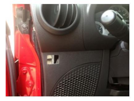
Drill a pilot hole in the middle of the area to be cut out. An air-saw is an excellent tool to use for making precise cut. You can also use a Dremel or other rotary cutting tool, but be aware it will create heat and melt the plastic around the cut line.
