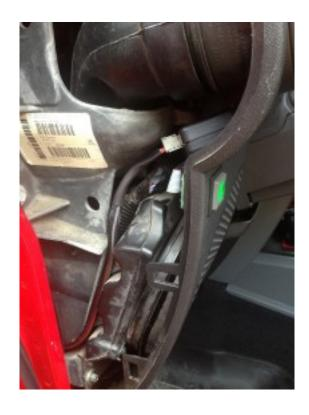
Tuck the interface module behind the dash and secure the wire harness neatly out of the way.
