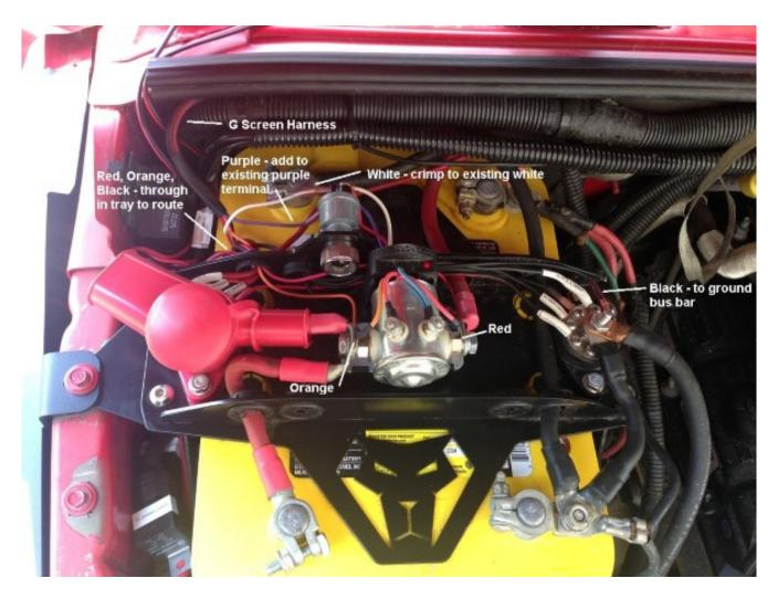
Route the wire harness across the engine compartment to the driver's side. Below the brake fluid reservoir there is a large rubber grommet. Cut a small slit in the rubber grommet to allow the wire harness through the firewall. Be careful not to damage any factory wires.
