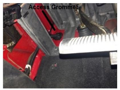
Open the driver's door and look up at the firewall above the brake pedal.
