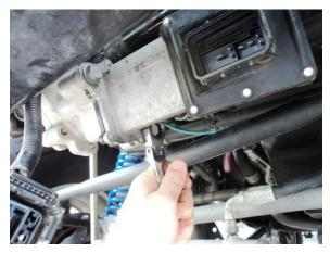
3. Remove factory swaybar actuator.
