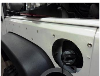
9. Install nutsets into drilled holes. Fully thread the long ¼" bolt with nut into the nutsert as seen in photo. With wrenches hold the bolt stationary and turn the nut 2 - 3 turns making sure that the nutsert does NOT turn. (There are tools specifically designed for installing these nutserts. Please
