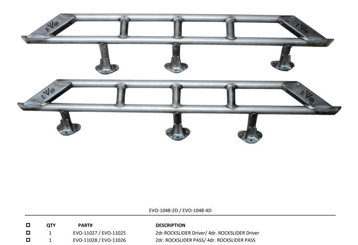
The EVO MFG RockSliders are intended to be welded onto your vehicle wherever you prefer, up if you have a body lift down if you don't, forward if you have large tires etc. This is one of the advantages of a weld-on slider other than their increased strength. Test fit sliders before painting or coating.
