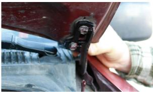
**3.** With the hood mounting bolts loose, slide the bracket forward or rearward as needed to give enough clearance between the bracket and the hood. In certain cases some trimming of the plastic cowl at the base of the windshield may be necessary to give the bracket adequate clearance. After enough clearance is achieved, align the marks made on the hood and the hood mounting brackets. Tighten down the hood mounting bolts.
