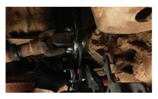
12. Install the (4) supplied M10x45MM long bolts and the (1) M10x100MM with the supplied lock and flat washers. Insert the supplied spacer between the back of the mounting bracket and the transfer case as shown. Once all the bolts are started into the transfer case, tighten the bolts to the appropriate torque spec as found in the vehicle's service manual.
