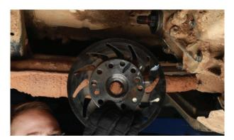
**4.** Slide the flange assembly onto the rear output shaft of the transfer case and apply Loctite thread locking compound to the output shaft threads. Reinstall the output flange washer and nut. Torque the nut to the appropriate torque spec as found in the vehicle's service manual. Stake the nut.
