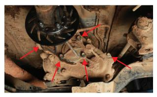
11. Take the caliper, E-brake arm, and mounting bracket assembly to the underside of the vehicle. With the whole mounting bracket on the transfer case side of the rotor slide the brake caliper over the rotor and then align the mounting holes in the bracket with the holes in the transfer case.
