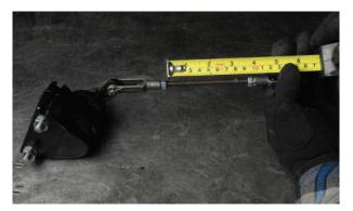
**9.** Attach the free clevis joint to the E-brake arm as shown. Slide the caliper into the mounting slots of the main mounting bracket. Loosen the lock nut on the adjustment screw of the brake caliper and then unscrew the adjustment screw until there are only a few threads of the screw in the caliper.
