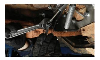
**16.** Remove the factory locking clip and E-brake pin from the factory E-brake mechanism. Remove the pin from the factory mechanism and then install the E-brake cable, pin, and locking clip onto the new E-brake arm as shown.
