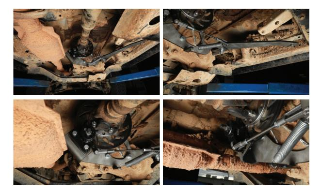
1. Disconnect the rear driveline by removing the (4) bolts holding the rear driveline to the transfer case rear output flange. Using a chisel, unstake the output flange nut. Loosen the output flange nut and remove the nut, washer, and output flange from the transfer case.
