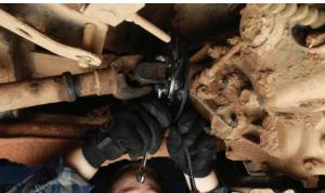
**6.** Bolt the E-brake arm to the main mounting bracket as shown using the provided 3/8" hardware and plastic spacer washers. It is important to place (1) plastic spacer washer between the metal 3/8" washers and the arm/mounting bracket. The remaining (3) plastic spacer washers should be installed between the E-brake arm and the main mounting bracket. Tighten the lock nut until the arm is snug against the mounting bracket but you are still able to rotate the arm freely.
