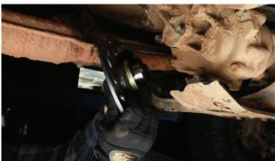
**3.** Ensure that the appropriate bolt pattern on the rotor and output flange are aligned. This bolt pattern will be the same bolt pattern used on the yoke of the rear driveline. It helps to mark the rotor and output flange at this point to make them easy to align later.
