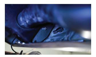
**23.** Install lower two mounting bolts, you will reuse factory hardware for this.
