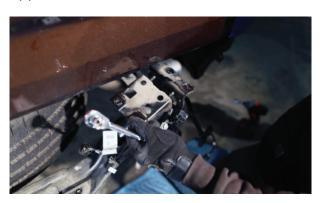
17. Install bumper mounts as shown using factory hardware and 2 5/16" bolts per side.
