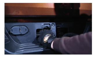
**3.** Remove 8 lower plastic pins and bolts on either side of the bumper.
