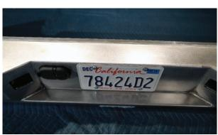
**20.** When installing trailer wiring connector pry up on metal clip from the rear until it snaps into place. We used a flat head screwdriver for this. The trailer wiring mount on the bumper is thicker than factory so this may take some effort.
