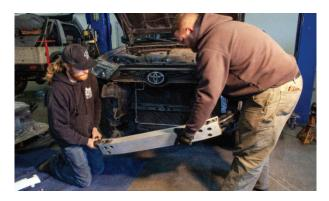
**12.** To aid in installation it is recommended to install two of the crash bar bolts from the rear of the vehicle, this will allow you to rest some of the weight of the bumper on the vehicle when installing.
