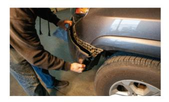
**7.** Once the bumper is removed separate the upper portion of the grill from the bumper.
