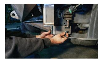
**18.** Before tightening the mounting bolts adjust the bumper so that there is approximately ½" -3/4" clearance between the bumper and the headlights. To prevent rubbing when the body flexes.
