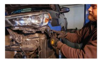
**10.** Reinstall the upper portion of the grille onto the vehicle.
