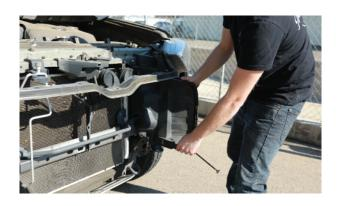
**9.** Remove the front bumper clip assemblies on both sides.
