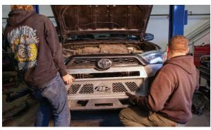
**15.** While someone is securing the bumper remove the bolt you installed in the front so that you can install the line guards. Repeat on opposite side.
