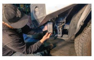
**16.** Remove bolts you previously installed from the rear of the bumper to aid install. And install them in the remaining holes.
