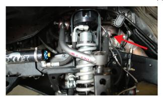
**4.** Slide the upper control arm bolt through the holes in the front and rear brackets as shown. Make sure to orient any washers and spacers previously used for mounting the upper control arm in the same way when bolting the brackets to the shock tower. See photos for reference.
