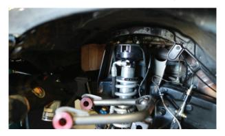
**12.** Reassemble the upper control arms with new bushings if needed. Grease the control arm bushings, inner sleeves, and the insides of the brackets. Reinstall the upper control arm and upper control arm bolt.
