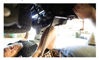
**3**. Near the top of the bumper mounting brackets are factory hangers that will hang on the pins in the frame. To remove the bumper, the bumper will need to be pushed straight up approximately <sup>3</sup>/<sub>4</sub>" before it can be slid back.
