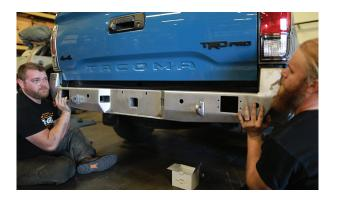
**13.** The electrical connectors can now be reconnected. You can wire the flush mount LED into the reverse lights or they can be wired separately on their own switch.
