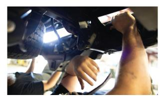
**2.** Loosen and remove the 5 mounting bolts on each side of the bumper. It is OK to remove all of the bolts as there are hangers that hold the bumper on for installation and removal.
