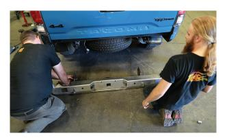
**12** . Install and tighten mounting bolts. Be sure to align bumper with the body at this point.
