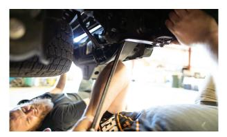
**5.** Disassemble factory bumper to remove wire harness, backup sensors (if applicable) and reverse light.
