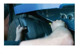
**15.** Remove two bolts holding PS cooler in place.
