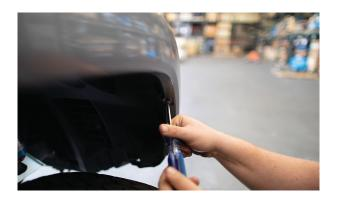
**6.** Mark around bumper mounting tab. **Do not cut this off**. This tab will help secure the remaining bumper. Your cut line can be slightly lower than what is shown in the photo, but no higher.
