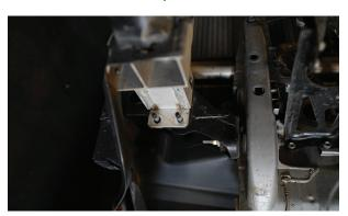
**13.** Remove bumper sub structure. It may be necessary to use a mallet or pry bar to remove.
