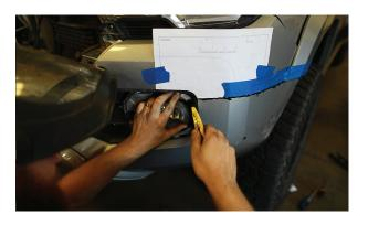
**10.** Remove clips and screws on lower portion of the bumper.
