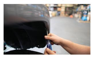
**23.** Center bumper with the body and tighten bumper mounting nuts. Reuse factory hardware.
