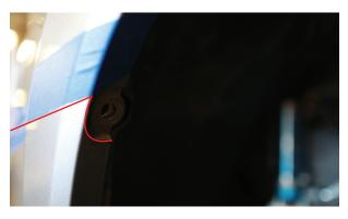
**8.** Cut around top of fog light using a utility knife.
