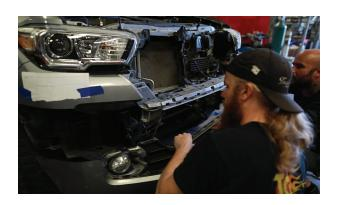
**12.** Unbolt the bumper substructure.
