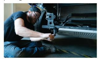
**19.** Before installing new bumper you can apply painters tape to help prevent and damage to vehicle finish.
