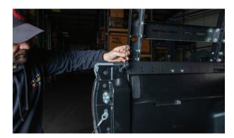
**2.** Remove the upper and lower taillight mounting bolts using a 10mm wrench or socket.
