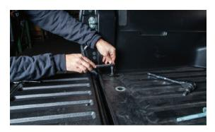
**5.** Remove the bed mount bolt as shown using a T55 Torx bit.
