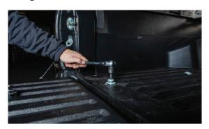
**6**. Set the new bracket in place and align the bottom mounting holes of the bracket with the holes in the bottom of the bed. Note the brackets are side specific, with the whip mounting tab oriented toward the front of the vehicle. Install the provided 7/16" bolt and washer on top of the bracket with the factory tie down mount. Reinstall the factory washers and spacers from the factory tie down mount underneath the bracket in the same orientation they were removed.
