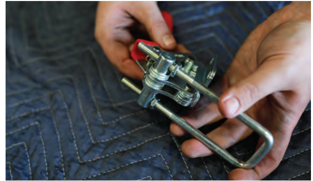
Insert the U-bolt through the rounded end of the swivel bar.
