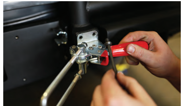
Hold the assembled latch up to the swing arm and begin to add the bolts as shown. Once properly aligned, torque all four bolts to 18ft-lbs.
