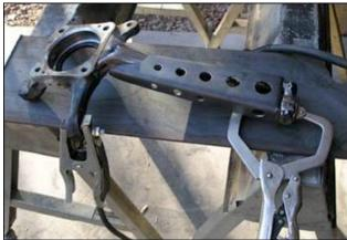
Tack the gusset to the spindle (left photo) Pictured on the right below is the finalized weld
