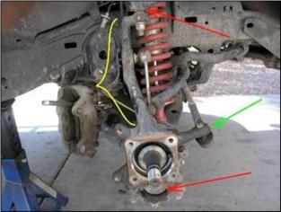
When disconnecting the sway bar link, inspect them for damage such as bending as pictured at the arrow below, or leakage from the boots. If you find damage, now would be a great time to upgrade to the All Pro heavy duty sway bar links and the sway bar centering collars we offer to prevent the problem from happening again.
