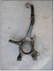
Finish disassembly and remove the spindle from the vehicle. Here is the knuckle, taken down to where nothing else is attached other than the grease seal that the axle rides in
