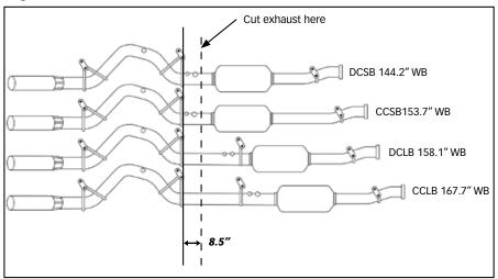
**5.** Remove the factory tailpipe from the vehicle by disengaging the exhaust system hanger pins from the rubber hangers using a large screw-driver or pry bar.
