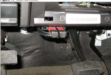
Figure 11 OBDII Connector
