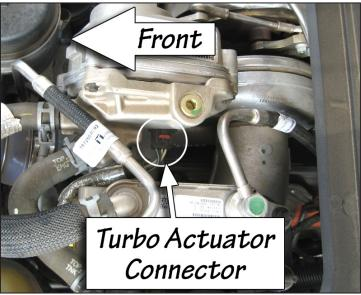
Figure 4: Turbo Actuator Connector
