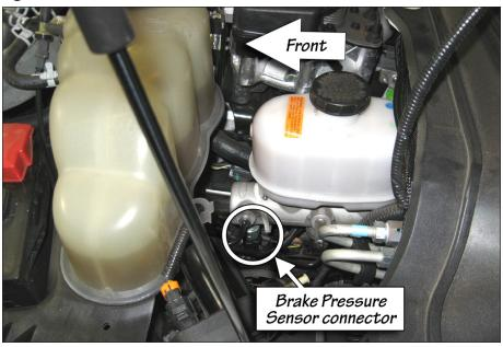
**6.** Locate the Banks Brake Wire Harness and connect the 2-pin male connector on the Brake Pressure Sensor harness to the 2-pin connector on the Banks Brake wire harness.
