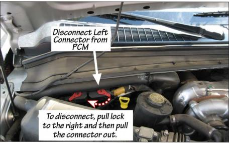
NOTE: Do not connect the Six-Gun PCM harness to the tuner. It will be connected in **step 17**.
