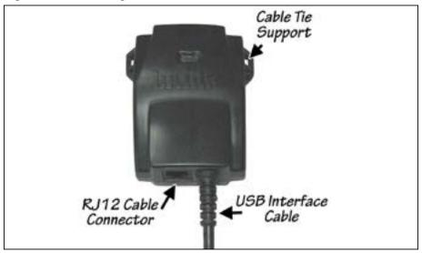
**11.** Route the Banks iQ USB interface cable from the Banks iQ Bridge Module under the dash and out through the fuse access panel opening. The cable can be slid under the door frame's seal and run up to the top of the dash. Pull enough cable to reach the Banks iQ and connect it to the USB receptacle on the left side of Banks iQ. See **Figure 8.** Snap the fuse access panel back in place making sure not to pinch the wire.
