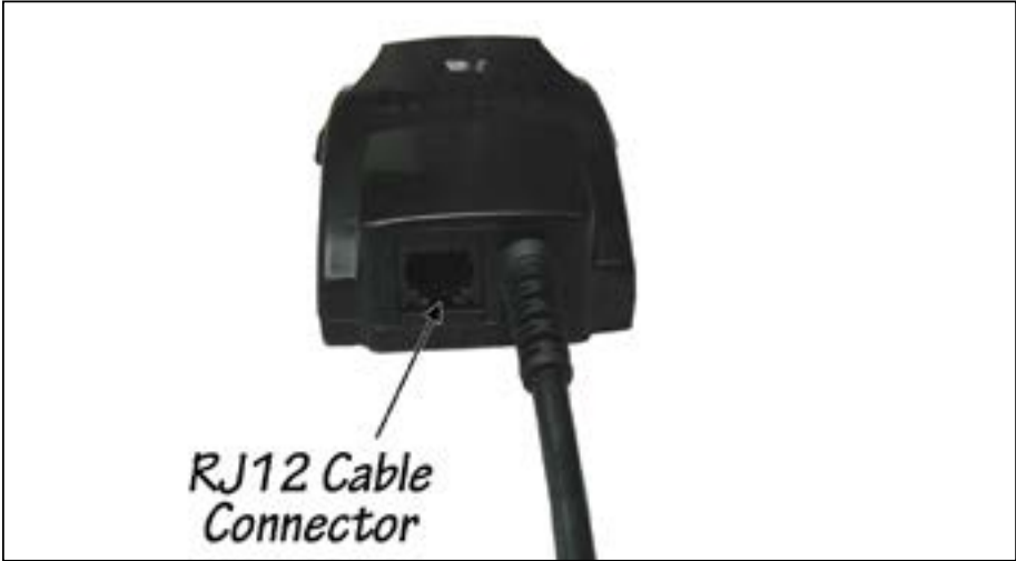
Figure 9 Banks Bridge Module
