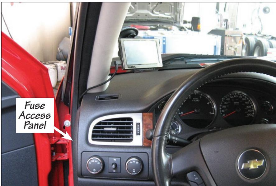
**7.** Locate the Banks OBD II Interface Cable in your kit. This cable has three connection points. Connect the RED OBD II connector on the Banks interface cable to the vehicle OBD II connector. Use a cable tie as shown in **Figure 41** to secure the Banks interface cable to the vehicle OBD II connector. Next, connect the 6-pin connector on the Banks OBD II interface cable to the 6-pin connector on the EconoMind Tuner harness.
