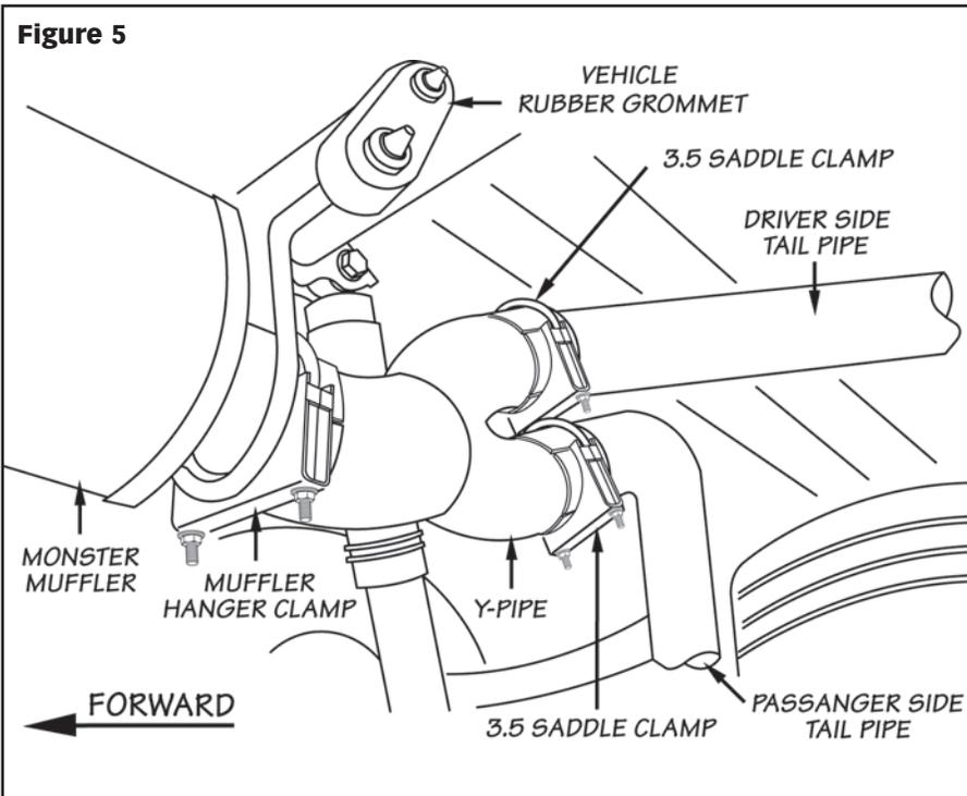
**13.** Insert the intermediate pipe inlet onto the flanged intermediate pipe outlet. Install the intermediate pipe hanger pin(s) into the vehicle rubber grommets.
