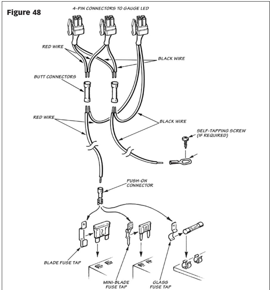
5. Connect the 4-pin connector of each gauge into the back of its corresponding gauge.
