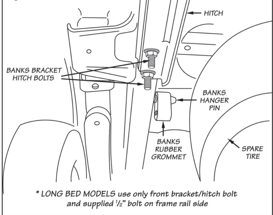
*For Long bed models, use one (1) bolt on the flat of frame rail and one (1) bolt on the side of the frame rail.*
