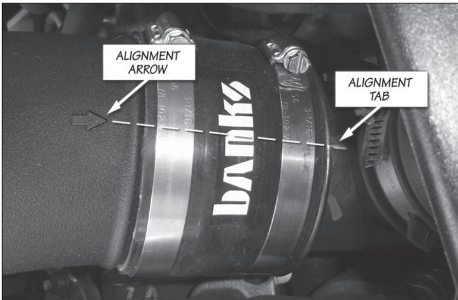
**21.** Now with the Banks Ram-Air filter housing cover and Banks bellows fully seated flush, fasten the Banks cover to the Banks housing using the Banks cover screws and tighten.
