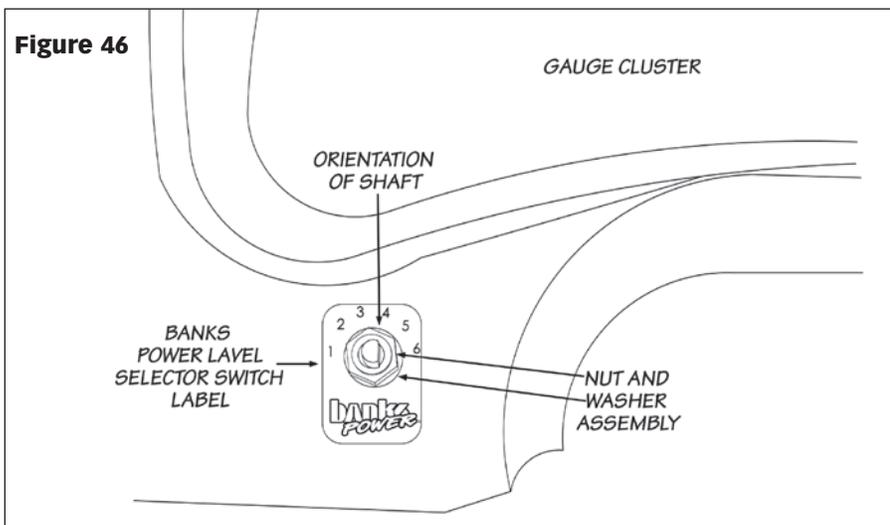
Snug the washer; be careful not to over torque the nut and damage the plastic threads.
