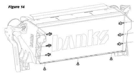
**15.** Install the trimmed front air intake shroud onto your Banks Techni-Cooler, using the six supplied push pins, and ratchet fasteners. *Figure 14*
