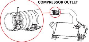
Figure 11c Clamp Assembly Positions Both Sides Lower
