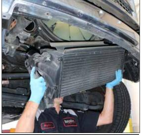
**6.** Loosen the upper clamp bolts on the right and left boost tubes and remove them from the vehicle. These will be replaced by the new clamps in your Banks Techni-Cooler kit. *Figure 6*
