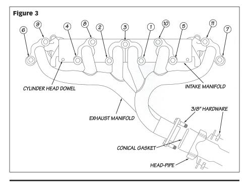
**13.** Install bolts 1, 2, 4 and 5 about three turns into engine block. Guide the intake manifold onto the cylinder head dowels. Loosely install all remaining intake/exhaust factory bolts. Be sure Banks TorqueTubes and intake manifold seats flush as bolts are tightened.
