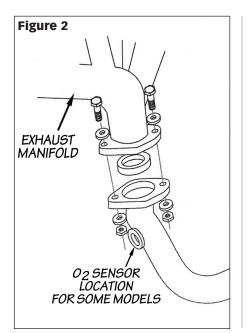
**9.** Remove the intake manifold from the engine block. Remove the remaining bolts (bolts 3,6 and 7) and remove the exhaust manifold.
