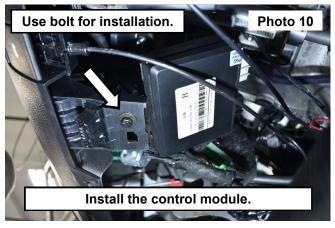
with the module tilted up. Use the supplied bolt to install. See Photo 10.
