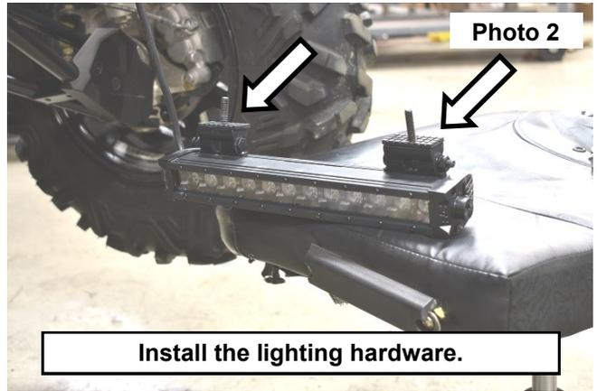
3. Install (2) of the supplied brackets onto the rubber mount and over the studs. Using the supplied nuts, snug the mounts on the light bar facing the front of the light. **See Photos 3 and 4.**
