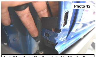
Install bracket with clip nuts behind fender liner.
