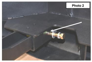
Install the supplied 1/2" x 3 1/2" bolts in the frame bracket as shown with the flat washers and lock nuts. See Photo 3.
