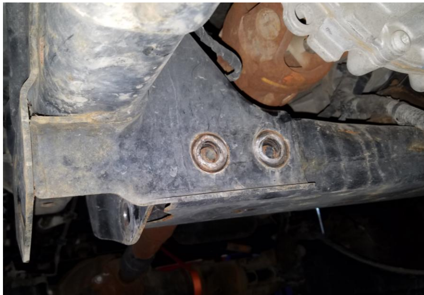
Figure 2. Transmission cross member bolts reversed
