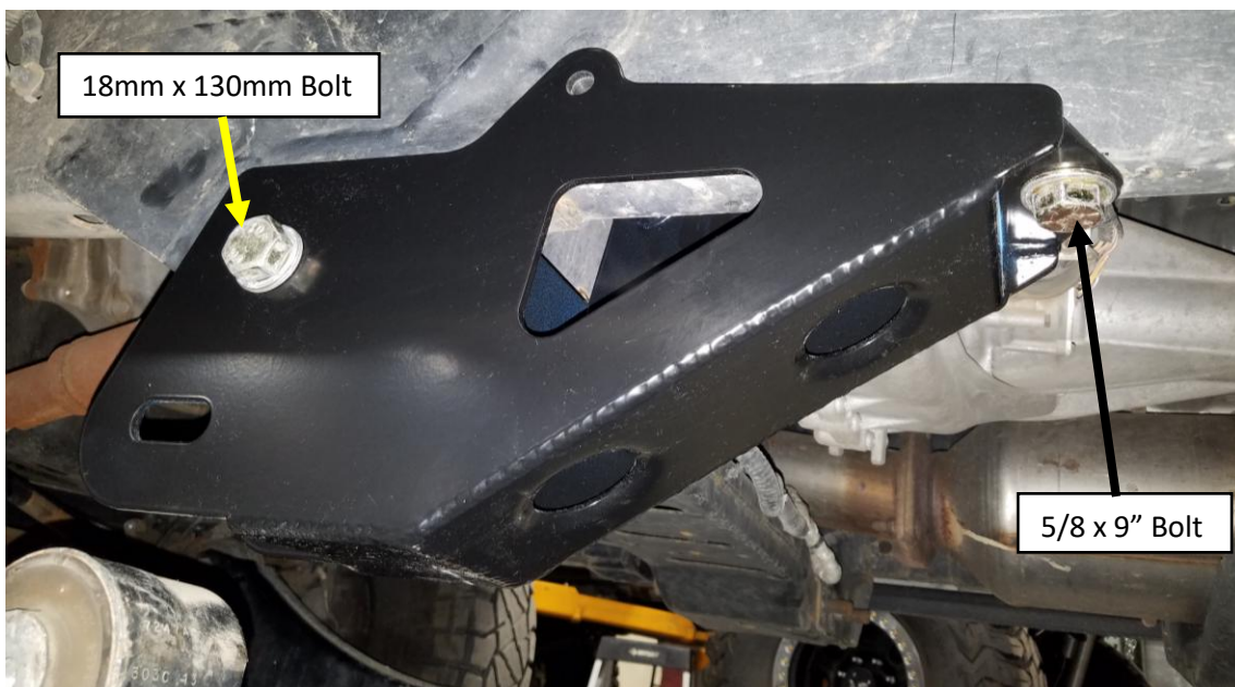
Figure 4. Synergy radius arm drop bracket initial install.
