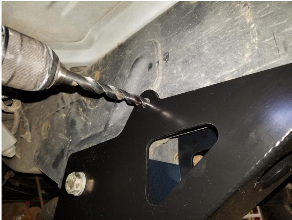
Figure 6. Using a drill to mark hole locations.
