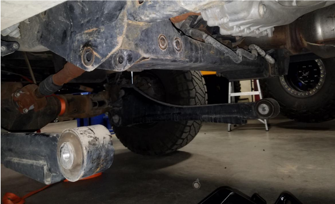
Figure 3. Radius arms separated from frame.
