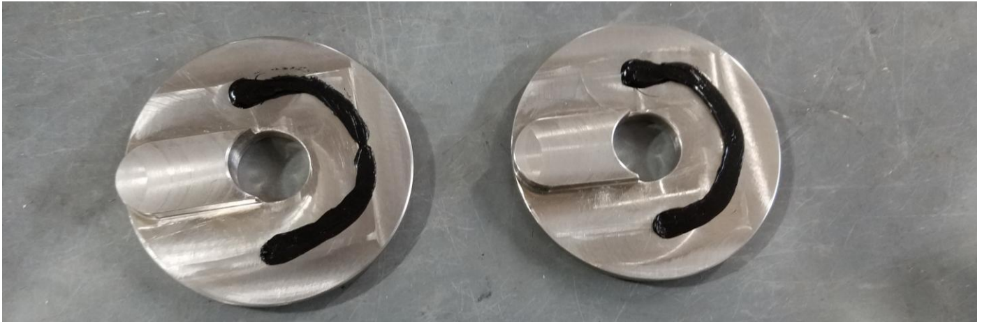
Figure 9. Sealant applied to spacers
