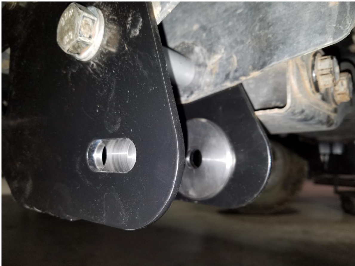
Figure 10. Radius arm position spacers installed.
