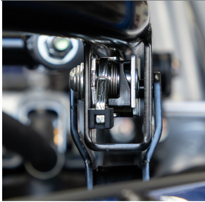
Figure 16: Latch correctly centered on striker frame.
