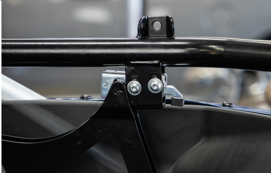
Figure 17: Latch Correctly Installed
