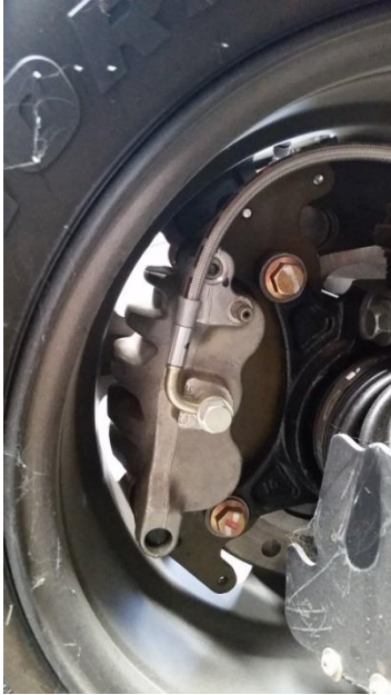
Figure 3: This is stock. The brake line fitting is far from the bleeder screw, this kicks the brake line up close to the wheel.
