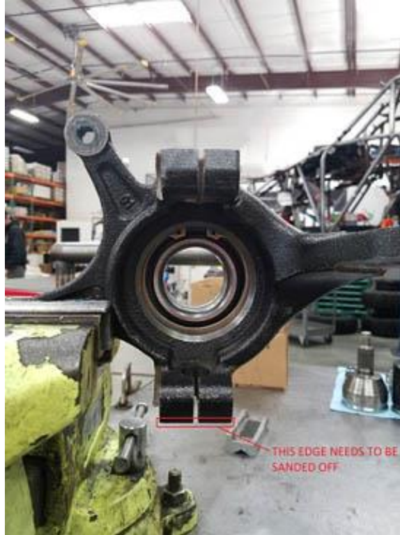
Figure 1: Notes show the area that will need trimming.
