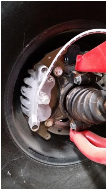
Figure 4: loosen the bolt a tad, just enough to turn the fitting closer to the bleeder as shown, retighten bolt.
